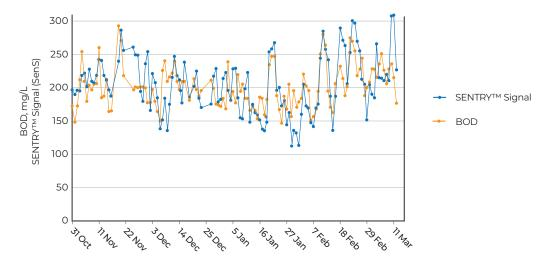
Real-Time SENTRY™ Signal (1440 points per day) compared with 5-day Lab Samples
