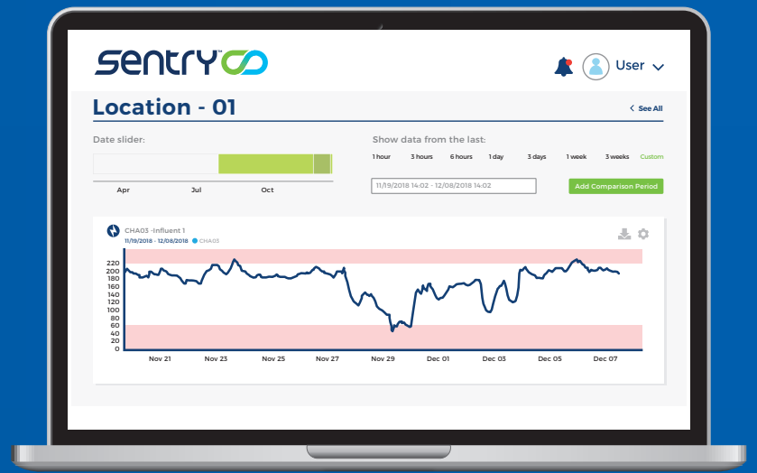
Real-time SENTRY data is sent to on-site SCADA & an online dashboard
